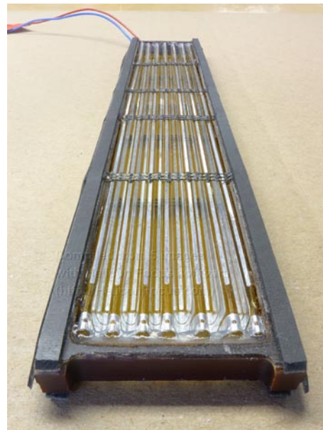
Diaphragm assembly of a ProAMT - the folded film can be seen clearly.
