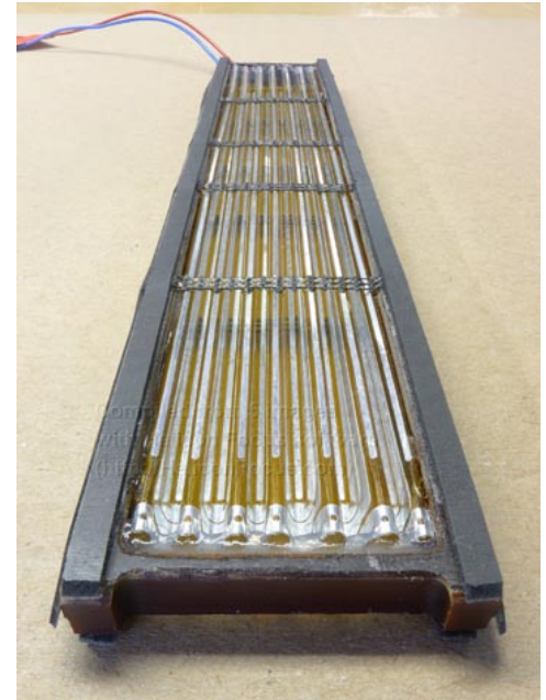
Diaphragm assembly of a ProAMT - the folded film can be seen clearly.
